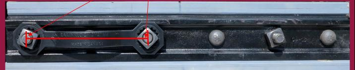
5.5-inch - designed to be on frog bars 2 1/8" (54 mm) hexagonal nut or or 2 1/8" (54.5 mm) square nuts.
